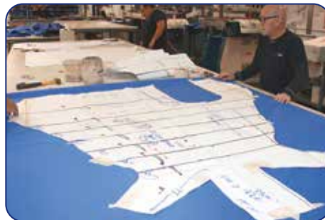
Sizing the material to the pattern
