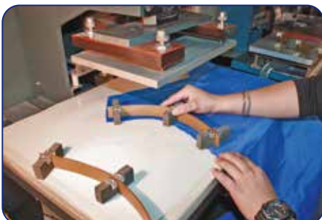
Custom fitting the RF sealing welds.
