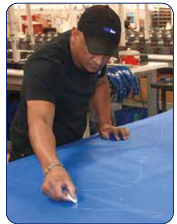
Transferring the pattern to the material
