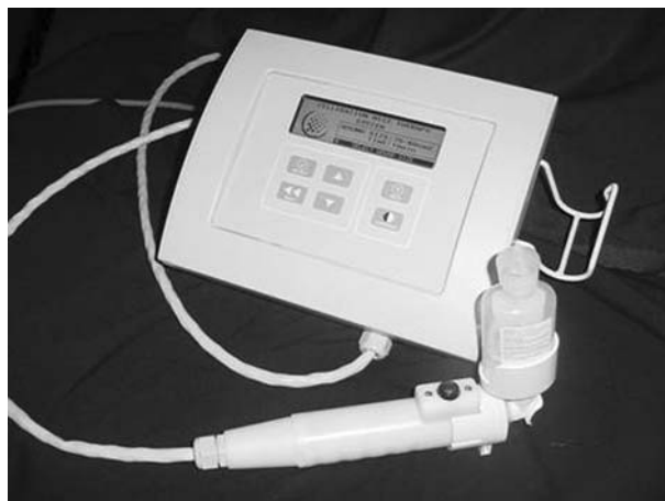
Figure 1. Noncontact low-frequency ultrasound system consisting of a generator, a transducer, and an applicator.
